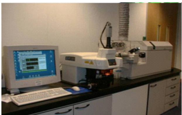
▶ *A laser ablation inductively-coupled plasma mass spectrometry instrument*
