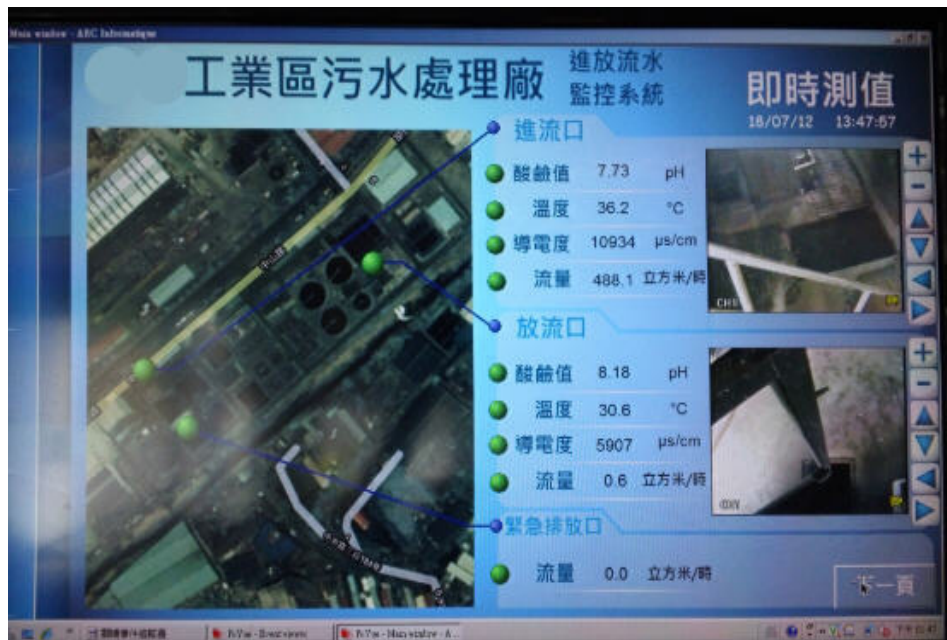
▶ Automatic monitoring system at the inlets and outlets of industrial wastewater drainage systems
