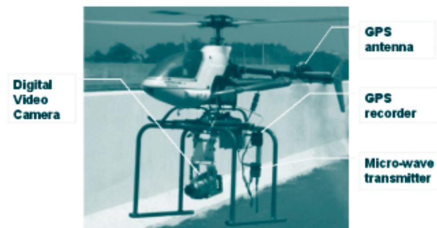
*Remote control helicopters are light and agile, and are equipped with a full set of precision instruments to gather evidence.*
