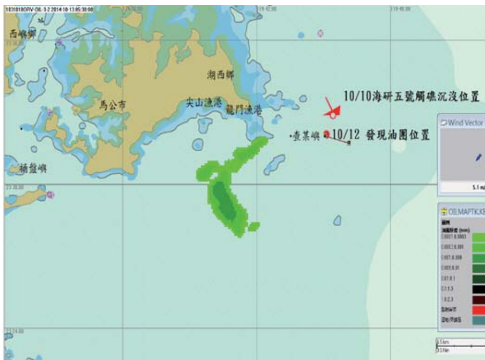
▶ Projected oil spill dispersal for 12 October 2014 in the sea surrounding the RV OR5 wreck site
