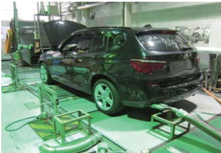
▶ Collecting and sampling vehicle exhaust for analysis
