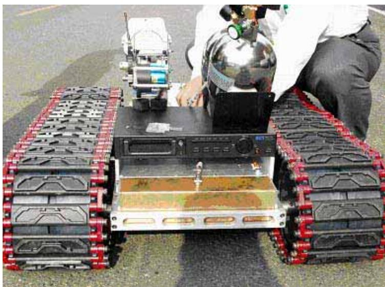
*Remote control detection and sampling vehicle*
