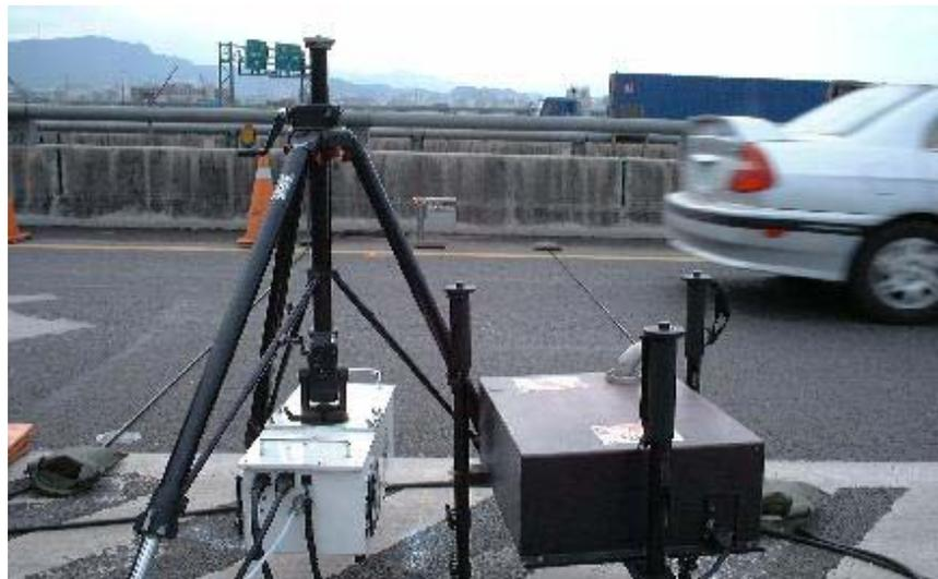
*Infrared remote sensing equipment in operation (photo source: EnviMac (榮諾科技))*
