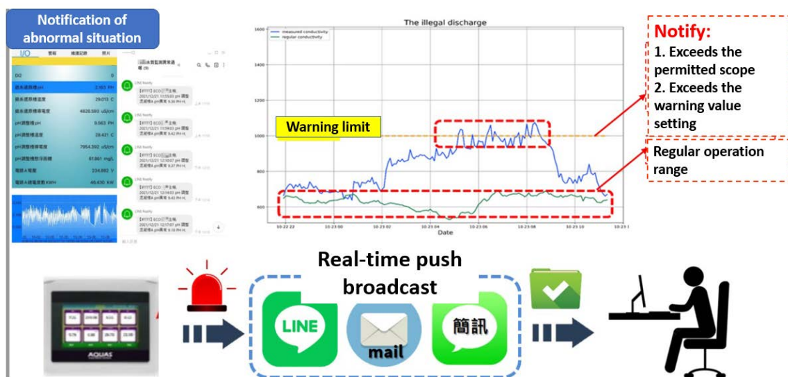
When an abnormality in water quality was detected, the equipment would send an early warning notification (through Line, SMS, or email)
