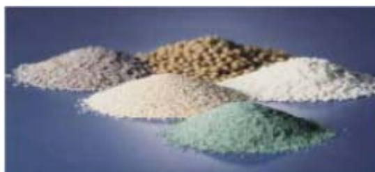
Fig. 2 Colorful crystals discharged from FBC system for treating different wastewaters.
